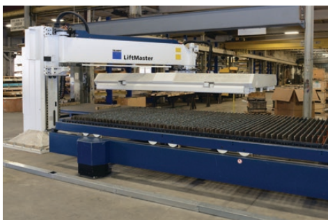
80" x 240" table offers the capacity to laser cut small or large parts
